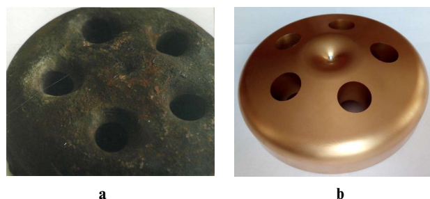
Fig. 1. The copper crown of the converter lance tip: a – the outer surface before operation; b – the outer surface after operation
