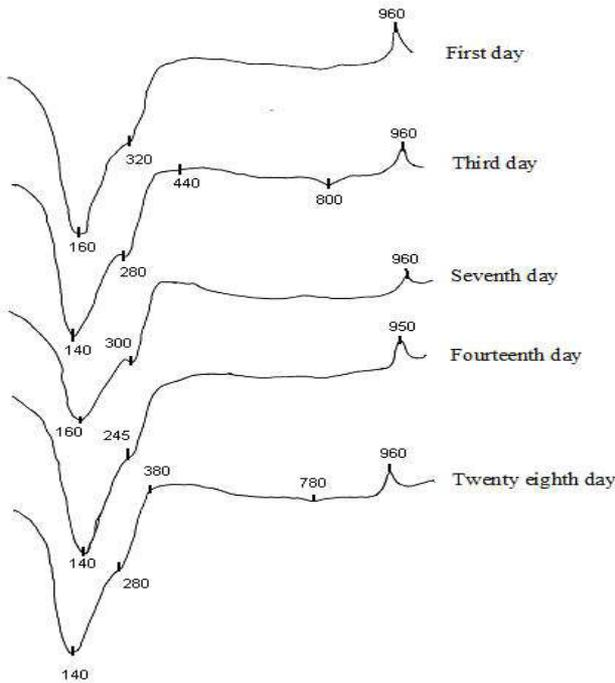
Fig. 1. DTA curves of hydrated alumina cement
